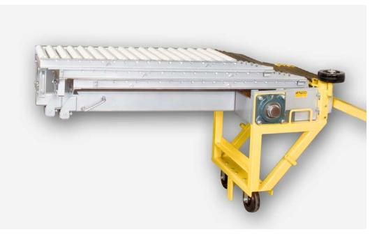
The Traversing Unloader is designed to assist the unloading of cargo and baggage containers and delivery trucks at a conveyor belt. It is mounted on t-rails adjacent to the conveyor to allow the unit to traverse to several different stations. The unloader telescopes, providing a roller conveyor surface for the unloading of containers or delivery vans.
