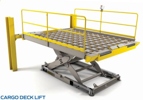
Adjustable height cargo deck designed to provide greater alignment of ULD dollies, trailers and dock heights, for ease in loading/unloading containers. Hydraulic lift ensures cargo is efficiently elevated to appropriate transfer height. Customized deck size is available with caster, ball or roller deck surfaces, to best fit the operation.
